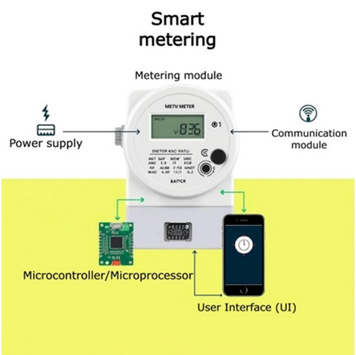
Figure 1: Key components of Smart meter
