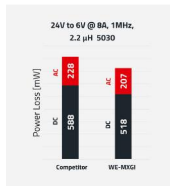
Figure 4 - AC and DC loss components of a 2.2 µH coil (WE-MXGI) in a buck converter with 24 V input, 6 V output, 8 A output current, and a switching frequency of 1 MHz, compared to another coil.
