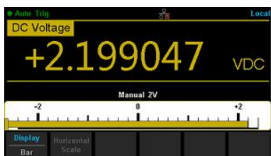
Bar Meter display mode adds a horizontal bar meter below the numerical display giving an analog indication of the measured value.
