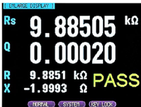
ENLARGE Display Enlarge Measurement Results and Include PASS/FAIL Result
