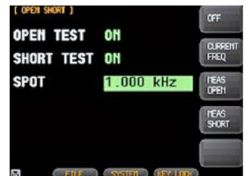
Selectable Fixture Zeroing Methods Full Frequency Range Zero or Spot Frequency Zero
