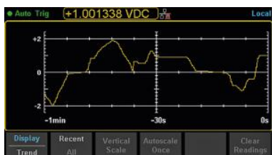
Trend Chart mode shows how the data changes over time in a value versus time strip chart display.
