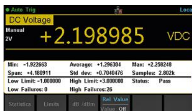
Statistics mode quantifies the data being captured whilst the Pass/Fail mode can quickly test, and instantly indicate if there is a problem.
