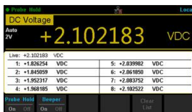
Hold mode provides a stable reading on screen even when the test leads are disconnected, enabling users to view the measured history data.
