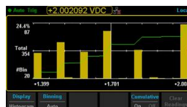
Histogram display mode shows how the data is distributed across a range of user defined Bin values.
