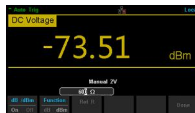
The dB and dBm functions allow relative measurements to either a stored relative value or 1 milliwatt depending on which function is chosen.
