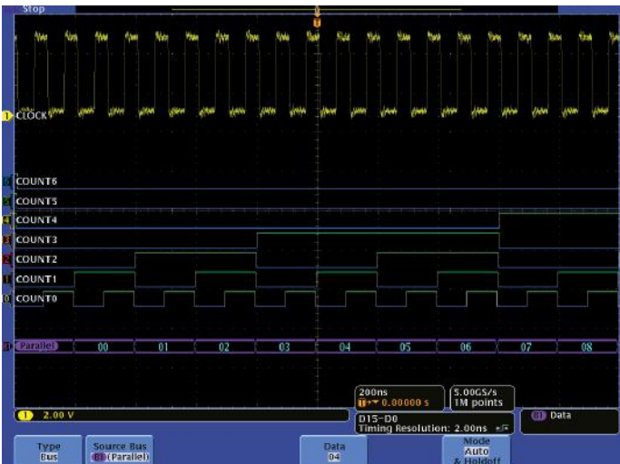
Figure 56. Automatically trigger, decode, and search on clocked or unclocked parallel bus data.
