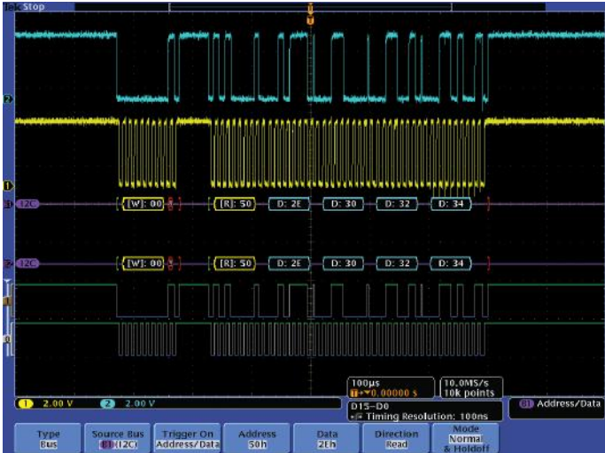
Figure 55. Serial bus analysis is accelerated with automated trigger, decode, and search on serial packet context.
