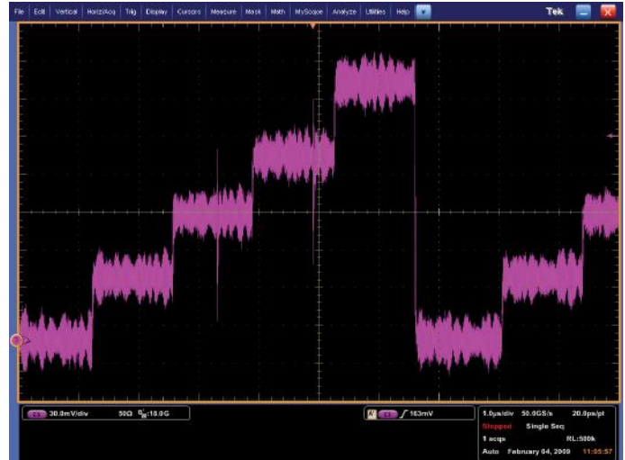
Figure 24. Peak detect mode enables the oscilloscope to capture extremely brief transient anomalies.
