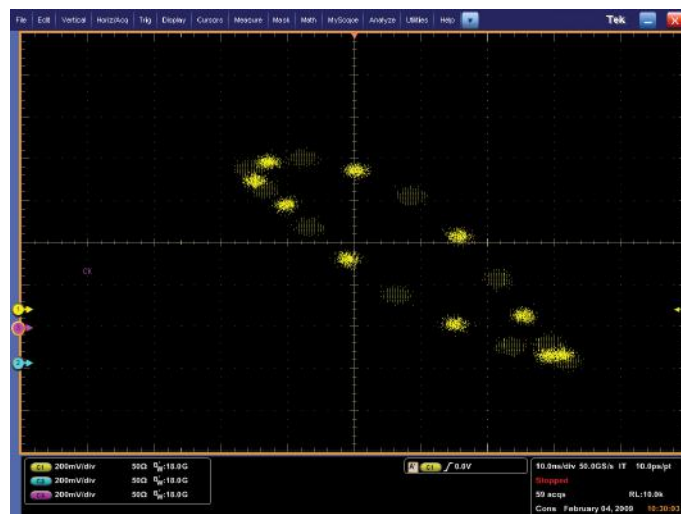
Figure 3. Two offset clock patterns with Z axis intensity grading.
