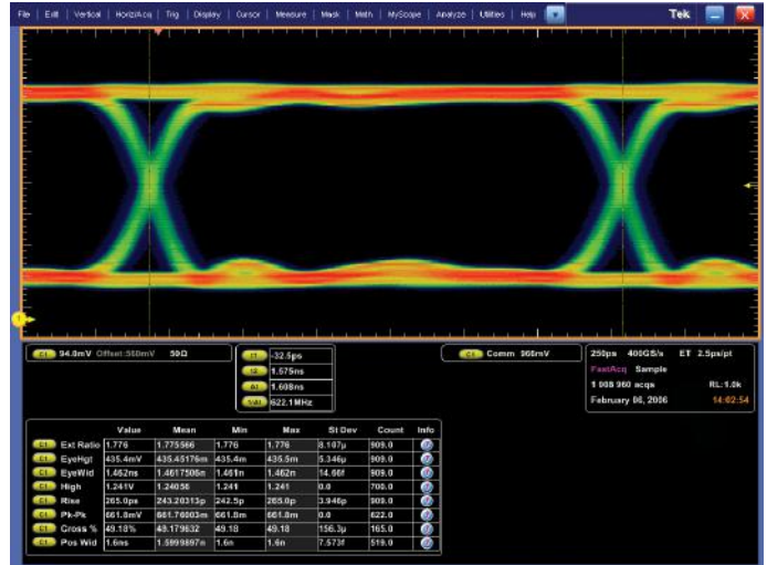
Figure 7. 622 Mb/s serial data eye pattern.
