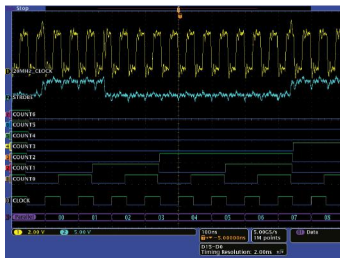
Figure 17. The MSO provides 16 integrated digital channels, enabling the ability to view and analyze time-correlated analog and digital signals.
