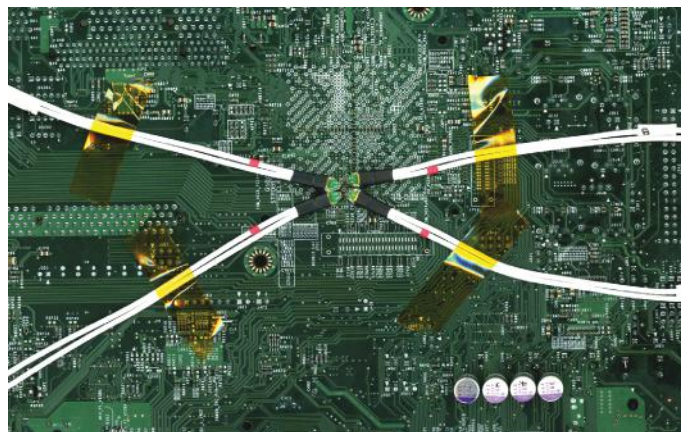
Figure 39. Dense devices and systems require small form factor probes.
