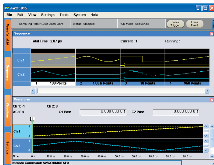
Figure 32. The Graphic editor and Sequence editor are combined for flexible waveform creation.
