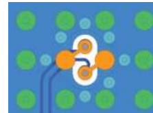
Initial Differential Via Design
