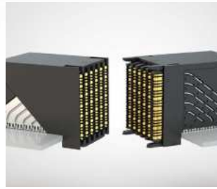
Coplanar available to bypass the midplane (EBTM-RA)
