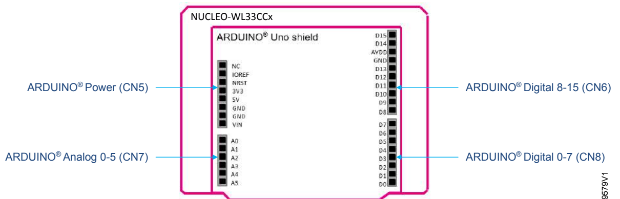
Figure 14. ARDUINO® Uno connectors and shield location
