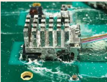
Expanded testing to MIL-DTL-55302 including salt spray and enhanced shock & vibration
