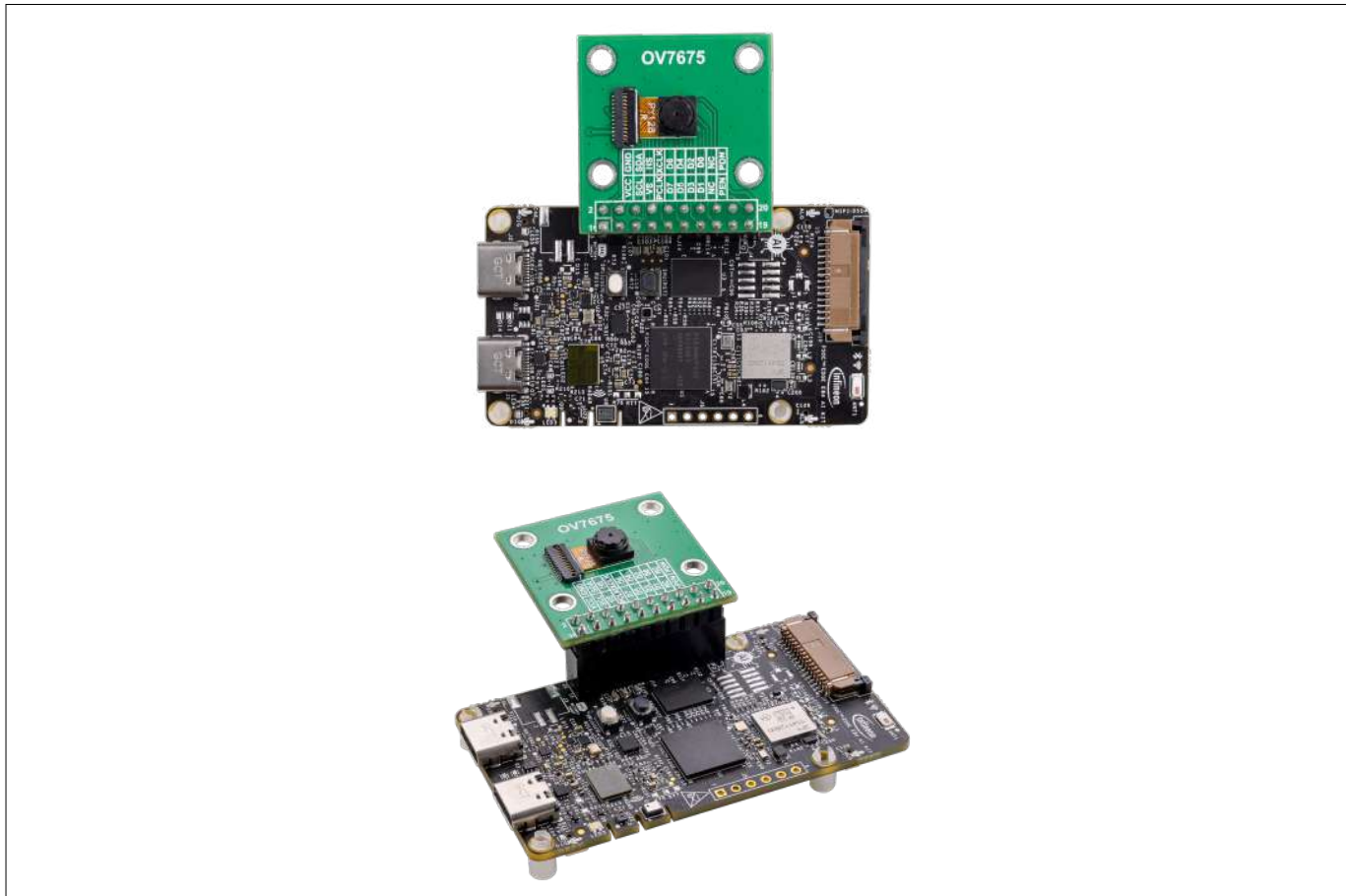
Figure 52 Connecting the DVP camera module to PSOC™ Edge E84 AI board
