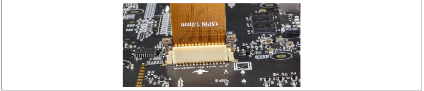
Figure 67 Connecting the MIPI DSI interface flex cable to 15pin FPC connector
